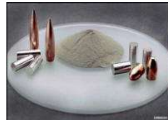
Frangible tungsten compressed bullets
