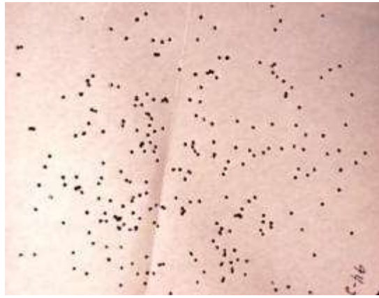
Witness panel fired into at a distance of 28 feet.
