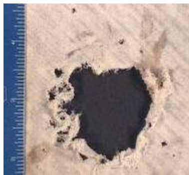
Individual pellets starting to break apart from the main mass of pellets.
