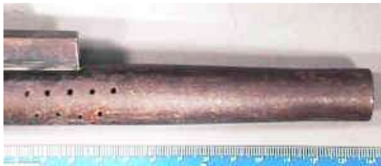
Barrel modified for use in a "Turkey-Shoot" competition. Extreme constriction or choke can be seen at the muzzle.
