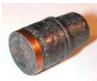
Gas-check copper base lead bullet
