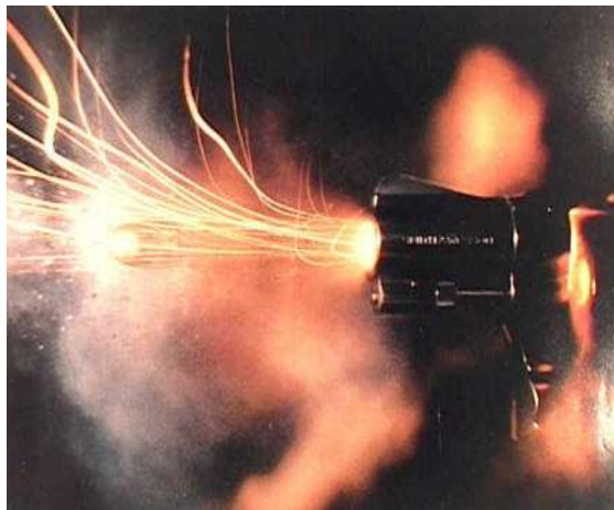
Time-lapsed image showing a bullet exiting from the barrel. Streaks of burning gunpowder, smoke, and unburned particulate can be seen exiting the barrel as well.
