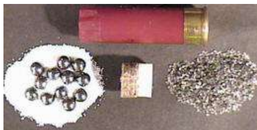
Components from a typical shotshell containing buckshot and a fiber/plastic wad combination.
