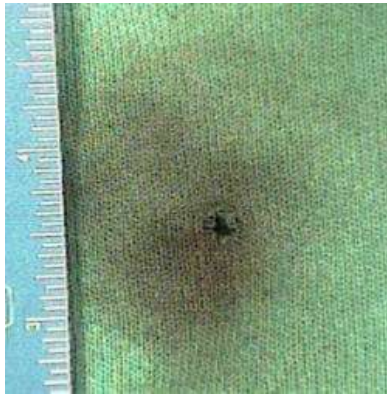
Visible gunshot residues around bullet entrance hole.
