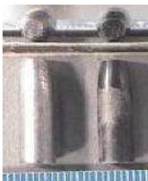
Steel cores from 7.62x39mm steel jacketed bullets
